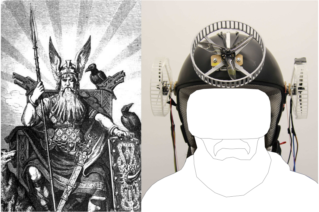
Fig. 2. Similarly to Odin replacing one eye and in exchange for knowledge, hence restricting his visual perception, the user trades the freedom of unconstrained head movement for the perception of simulated g-forces in VR. Odin's Helmet uses four propellers on each side of the device to simulate force as a modality for haptic feedback.
